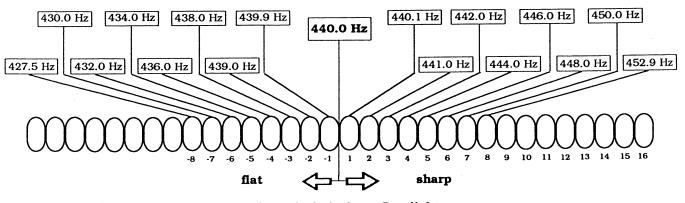
The pitch indicated in the boxes is the pitch at which the lamp first lights.
