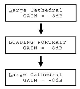
If the organ is equipped with a VDU, the VDU will also flash while the new pallet is loading. Once the newly selected pallet is loaded the display will change back to the Acoustic Portrait™ pallet name and the VDU will stop flashing.
