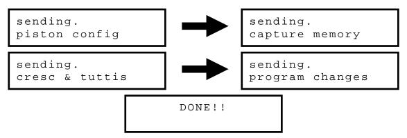
The 'dot' behind the word 'SENDING' on line one of the display will move as the data is transmitted.
