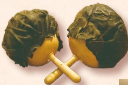
Ink balls were used to put ink onto the type.
