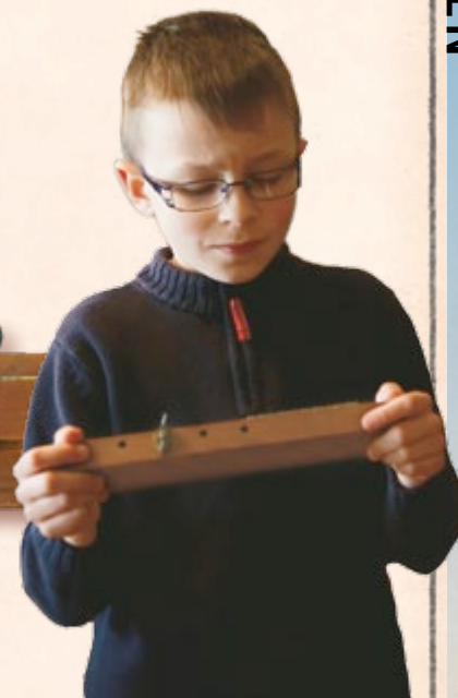
The typesetter had to place one letter at a time into an instrument called a composing stick.
